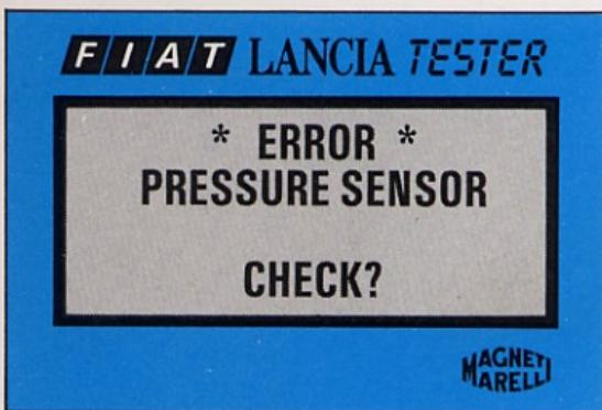
Upon pressing key **OK** guided diagnosis is entered, leading the operator to error identification.
