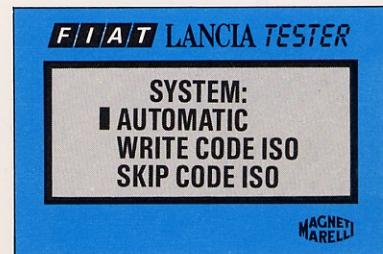
The operator can select the desired test program by means of **Δ** and **∇** and put it through execution by pressing key **ES**
